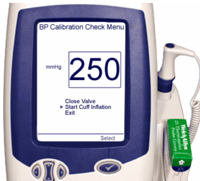
Figure 19. Fine Tune the Pressure Reading to 250 mmHg
